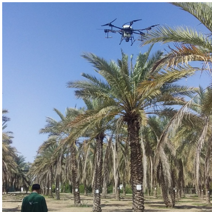
Liquid pollination through a drone also known as showering
