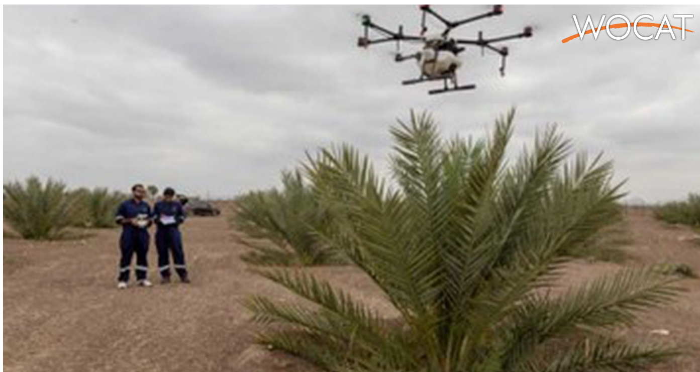
Palm tree being 'showered' i.e., liquid pollination by drone
