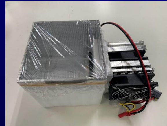
Water Harvesting Device from the Air with Metal Organic Framework
